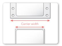
Width of the backing liner from edge to edge.
